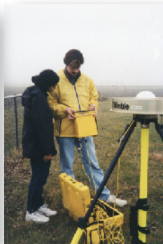
Summer intern Melvin Mattocks collects field spectra with a spectroradiometer.
