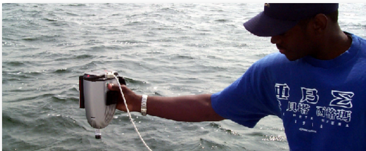
Summer intern Melvin Mattocks collects field spectra with a spectroradiometer.
