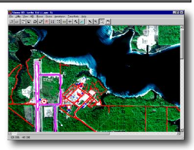
ERSC worked with Orbital Technologies Corporation (ORBITEC) to develop a real-time navigation system for airport emergency response vehicles. Above is a 4-meter resolution satellite image of Tyndall Air Force Base, FL with runways and access roads in a GIS overlay.
